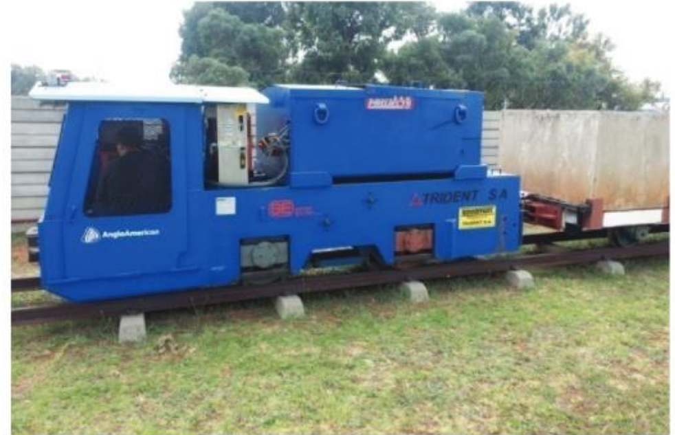
Figure 1. Fuel cell powered mine locomotive of Vehicle Projects Inc. utilizing the PEM fuel cell and reversible metal-hydride storage, currently being trialled at AAPL's School of Mines
