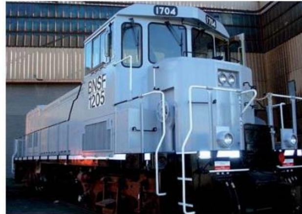
Schematic and picture of the fuel cell switcher being Developed by Vehicle Projects (picture courtesy of Vehicle Projects LLC)
