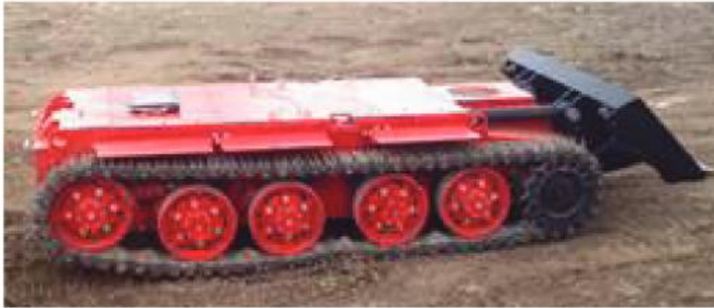
Figure 2. Fuel cell powered mine dozer, utilizing PEM fuel cell reversible metal-hydride storage, currently undergoing surface trials
